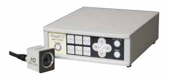
The MKC-310HD employs 3x 2.1Mega pixel Full HDTV 1/3-inch CMOS sensors to provide 1000 lines of high definition video images through 3G-SDI output interface, coupled with High Sensitivity performance of F10/2000 lux providing the optimal video quality required for special applications.
